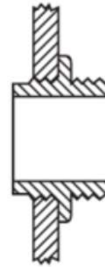
Outlet square and projecting into barrel (coef. 0.70)
