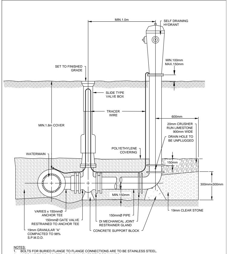
2. HYDRANT TO BE LOCATED AS SHOWN ON PROFILE DRAWINGS.
