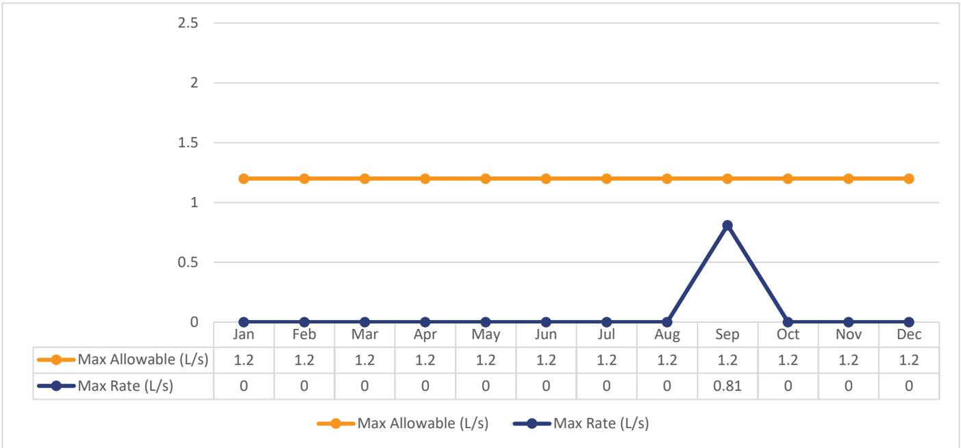
**Note:** Well #3 not in use following well casing collapse on September 28, 2023. In September 2025, the significant spike was due to annual calibration of the flow meter and did not indicate a true value. All spikes are reviewed for compliance with O. Reg. 170/03.
