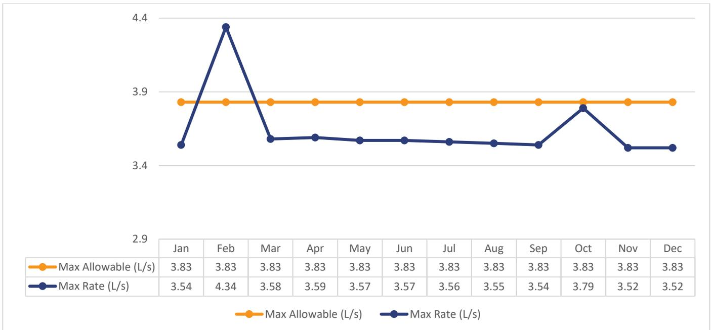
**Note:** Certain operational circumstances could cause results to be temporarily outside of the allowable rates. In February 2025, the allowable rate was momentarily surpassed due to a brief spike caused by well pump start up. All spikes are reviewed for compliance with O. Reg. 170/03.
