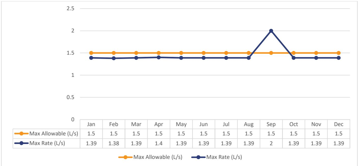
**Note:** Certain operational circumstances could cause results to be temporarily outside of the allowable rates. In September 2025, the allowable rate was momentarily surpassed due to annual calibration of the flow meter and did not indicate a true exceedance. All spikes are reviewed for compliance with O. Reg. 170/03.
