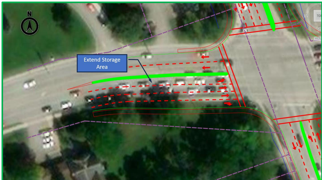
Figure 13: Extend Storage Area of the West Approach
