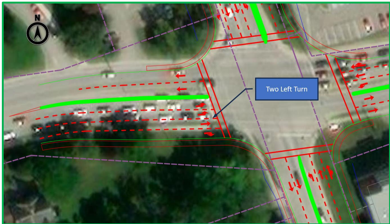
Figure 14: West Approach with Two left-turn Lanes
