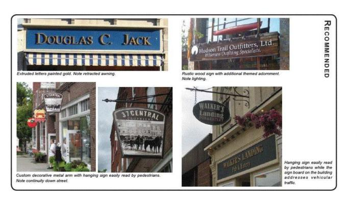
Historically, store signs were painted on a wood base, or made of raised wood or ceramic letters mounted on a wood base. Type face should be clear and easy to read. Painted plastic letters and moulded polyurethane signs can be used to re-create historical styles, while reducing maintenance. Stainless steel letters or similar alternatives are acceptable. Colours should be coordinated with building.
